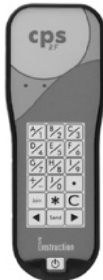
eInstruction’s radio frequency receiver (above) and response pad, or “clicker” (below).
