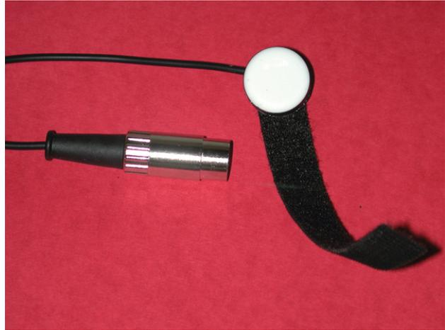
Fig 10.7. Pulse plethysmograph transducer.
