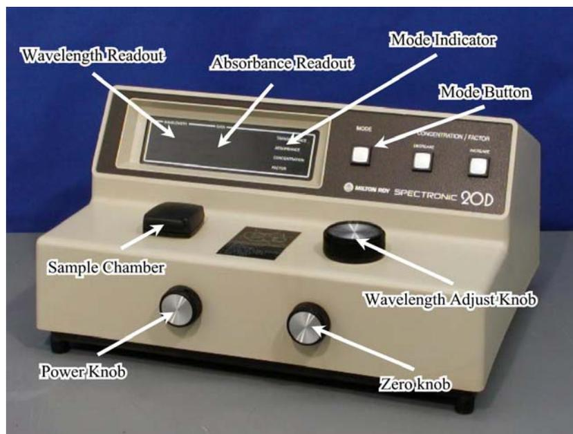
Fig 4.18. The Spectronic Spec 20 spectrophotometer.
