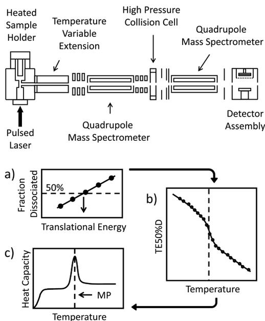
**Figure 1.** Upper half shows a diagram of the main components of the experimental apparatus. The lower half shows the main steps involved in measuring melting temperatures for size-selected cluster ions.
