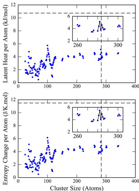
**Figure 4.** Upper panel shows the latent heat per atom plotted against cluster size for the measurements reported here (150–342 atoms) and from previous measurements for smaller sizes (24–128 atoms). The dashed horizontal line shows the bulk value, and the inset shows an expanded view around the jump in melting temperature that occurs between 283 and 284 atoms. The dashed vertical line indicates the location of the jump. The lower panel shows a similar plot of the entropy change per atom.
